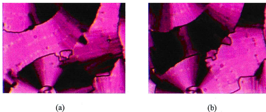
Figure 6(a, b). Photomicrographs of the optical textures of the two ferroelectric states in the ' B_7 ' phase of B-10(S) ( 149^\circ\text{C} ).
